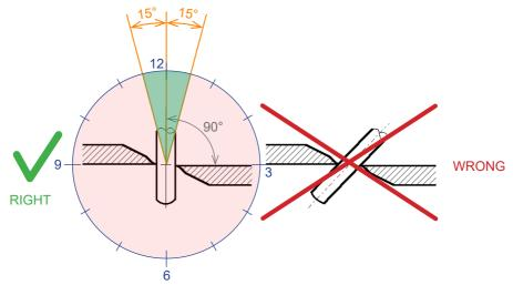
Higher cutting capacities can be achieved by cutting as close as possible to the blade's pivot point.
