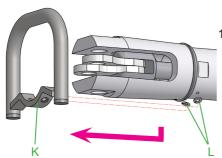
Take the handle 'K' away in direction of the lever elements and also remove the washers 'L' underneath.
