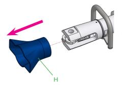
8. Finally, remove the protection hose 'H' from the tool as shown.
